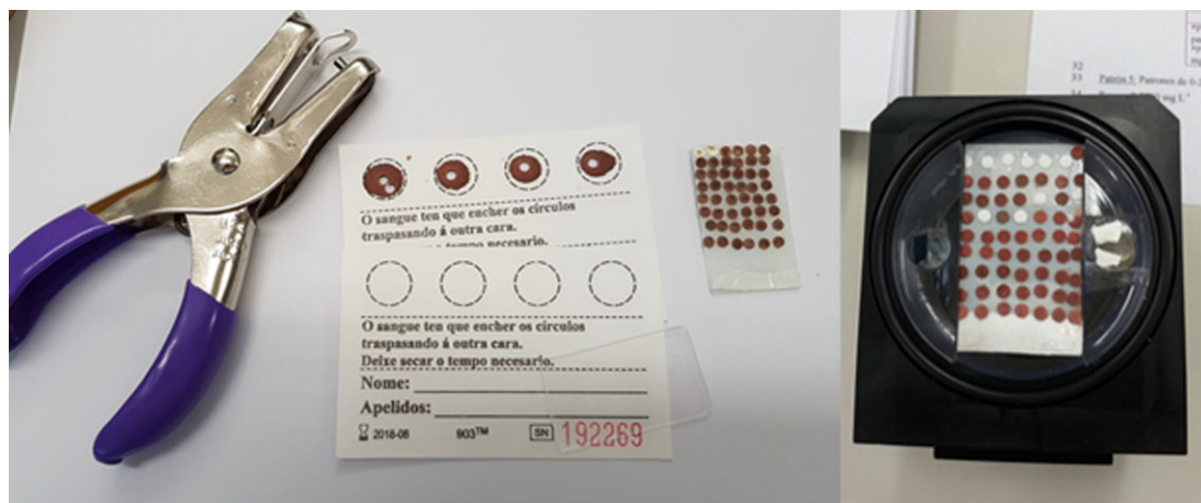
Fig. 1 Circular filter paper disks (3 mm) with DBSs from different real samples and reconstituted Seronorm CRMs.
